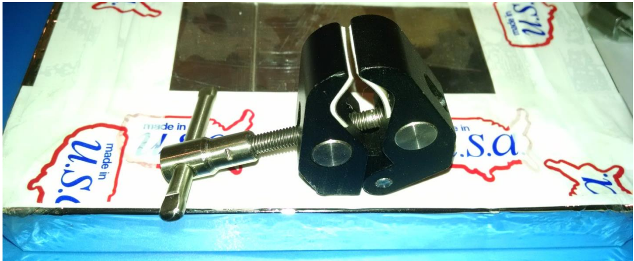
6) AFTER THREAD HAS REACHED BOTTOM, BACK-UP CLAMP UNTIL IS PARALLEL WITH MIRROR SIDE.
